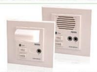
installed at bedside of a patient's bed to call a nurse, a patient can press a call by pressing a button at bedside or pressing button (NC64-BCC "accessory") at the end of the cord. A nurse can indentify where a call has come from (blinking light) without having to check with Smart Digital Console. A nurse can communicate with a patient (full duplex), the device comes in 2 models, single and double bed.
